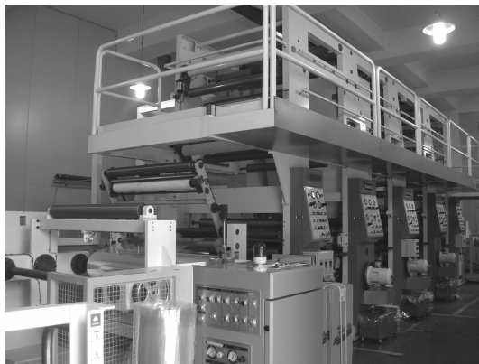
Fig. 7. Three-layer gravure printing machine.
